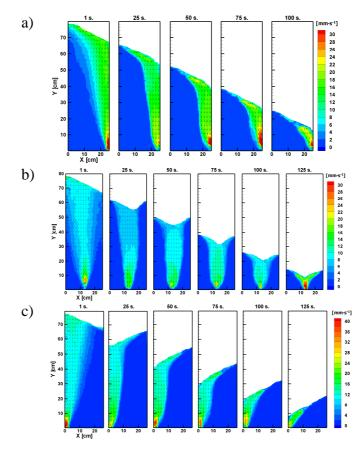
**Fig. 1.** Velocity contours for eccentric filling in the left part of the model and a) discharge on the right, b) discharge in the central line, c) discharge in the right part of the model
