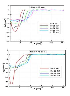
**Cont. Fig. 2.** Velocity profiles for the flow of flax-seed obtained for a) eccentric filling and discharge on the opposite side, b) eccentric filling and central discharge, and c) eccentric filling and discharge but on the same side of the model
